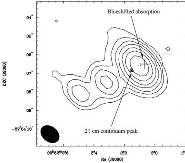
FIG. 1.—ATCA 8 GHz radio continuum image. The contour levels are 0.75, 1.5, 3, 6, 12, 24, 48, and 96 percent of the peak value of 163 mJy beam<sup>-1</sup>. Positions of the 21 cm continuum peak and of the H I absorption are marked with crosses, with sizes representing the 1  $\sigma$  error bar.
